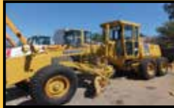
1 x Komatsu GD650 Grader with ripper 1 x Cheng Gong MG2320B Grader with ripper and cat 3306 engine
